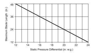
This damper's design at a blade length of 48" has a maximum allowable blade deflection of L / 360 for the static pressure indicated on the chart. At reduced blade lengths, higher static pressure limits can be attained without sacrificing damper operating and performance characteristics.
